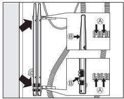
■ Secure the transit bars to the back of the washing machine. Make sure that holes (B) are fitted over retainers (A).
